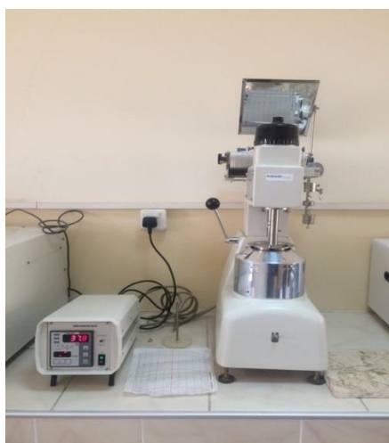
Figure 2. Amylograph, Brabender® GmbH & Co. KG Germany equipment used for investigating the effects of various ingredients, such as enzymes, on dough properties.
